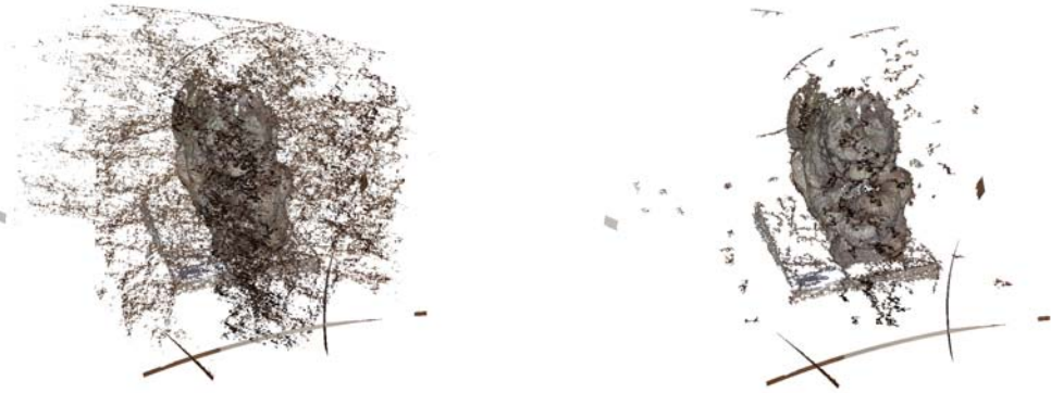
Figure 5: An example of the automatic filtering operation performed by the MeshLab tool. Small floating triangles caused by acquisition noise are automatically removed.
