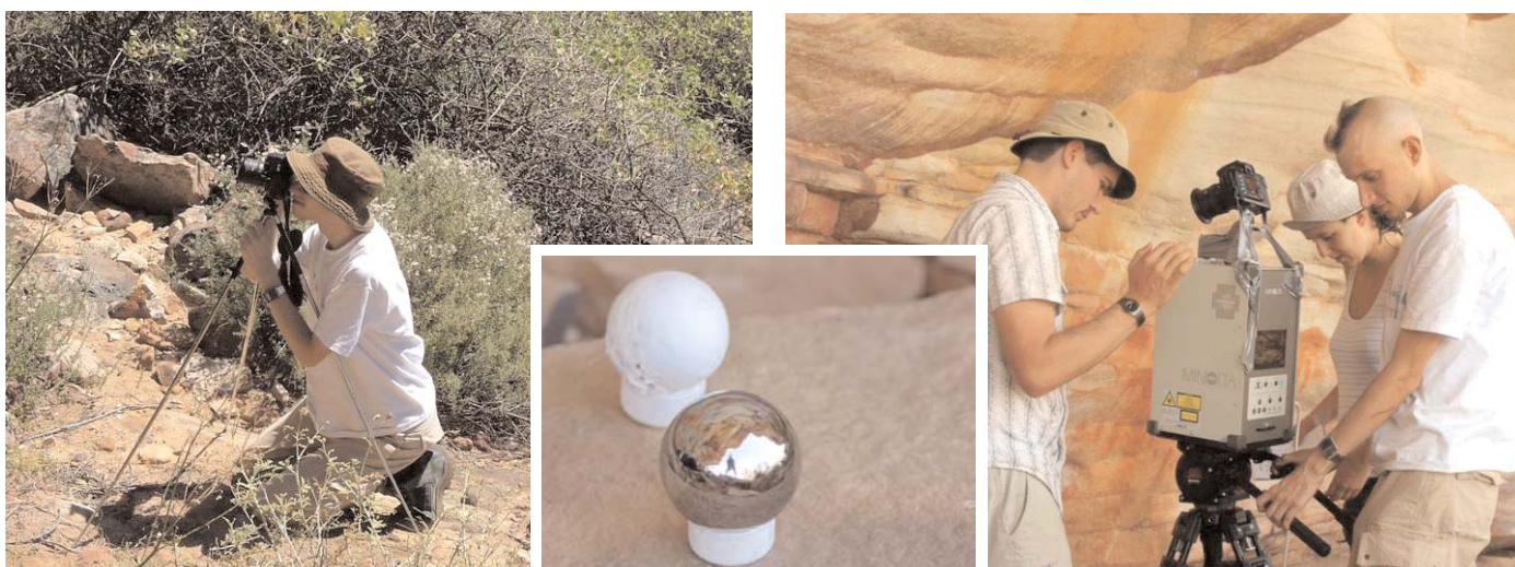
Figure 6:(a) Capturing detailed photographic record (b) Light probes (c) Laser scanning the site
