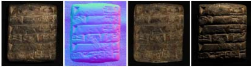
Figure 16: From left to right: One of 264 captured images of a cuneiform tablet; recovered normal map (colour coded in the usual way); recovered albedo map and a virtual re-lighting.
