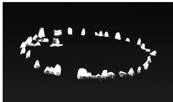
Figure 4: Long Range, Low Resolution Scan of Castlerigg Stone Circle. By Nick Rosser.
