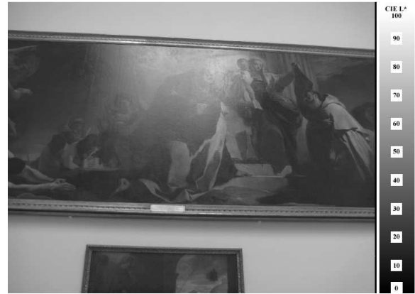
Figure 2: Grey-levels map of lightness values generated from data shown in Figure 1 using CIE L^* . The luminance factor in each pixel is given by the ratio between the luminance value and the maximum value of luminance in the scene.
