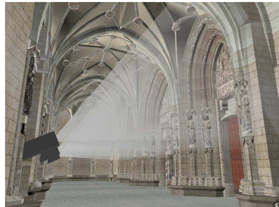
Figure 2: Interactive 3D application for studying projectors viewing the 3D model of the portico with three parallel projectors and their light beams.
