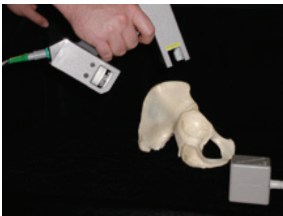
Figure 1: Polhemus hand-held laser scanner.
